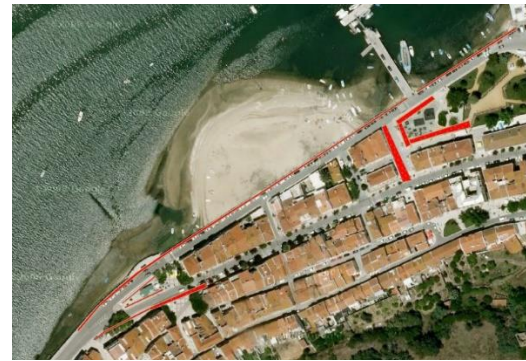
Figure 9 - Infiltration trenches technique applied in QGIS
